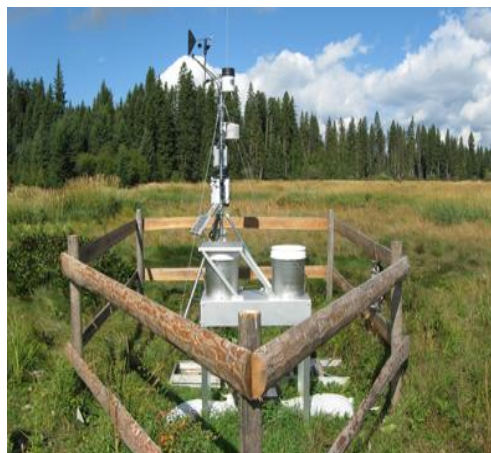
Figure 28. WLI Weather Station/Bulk Loading.
