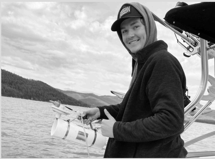
An Ashely Lake volunteer for the Northwest Montana Lakes network deploys a sampler to collect water samples from discrete depths.
