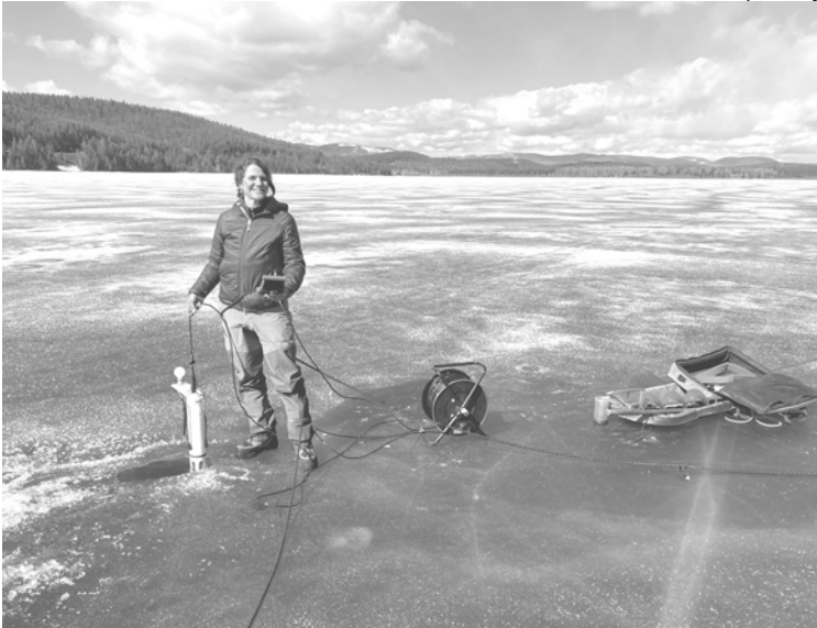
Durae Belcer lowers a Hydrolab which measures physical water quality parameters from the surface to the bottom of the lake.
