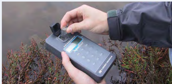
Fluorometer. Photo courtesy Whitefish Lake Institute
