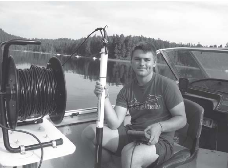
Summer intern Zach Cook prepares to deploy a data sonde to collect various water quality parameters.
